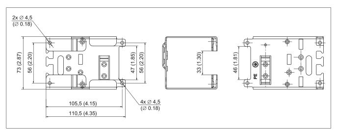
Figure 8-9 Dimension drawing of Screening Kit, frame size FSA, all data in mm and (inches)
