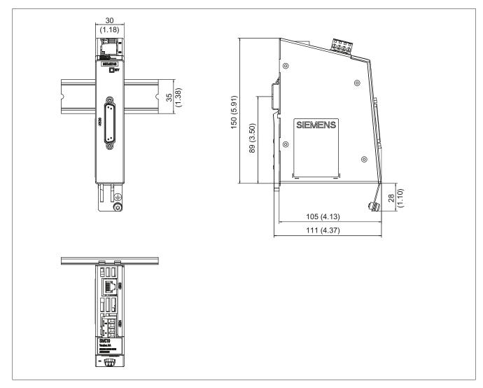
Figure 7-4 Dimension drawing of the Sensor Module Cabinet SMC10, all dimensions in mm and (inches)
