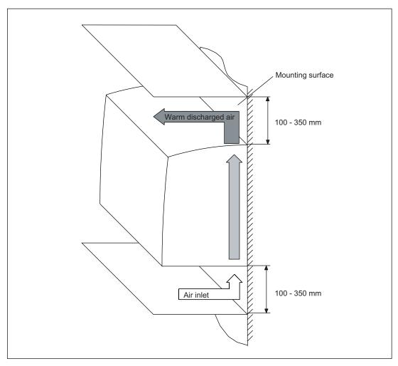
Figure 9-3 Cooling clearances
