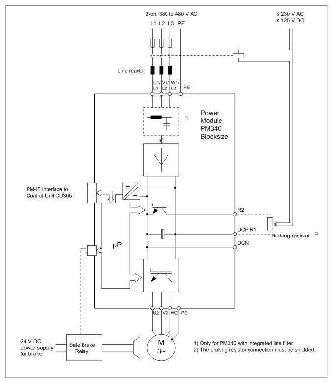
Figure 3-9 Connection example PM340, 3-ph. 380 V - 480 V AC
