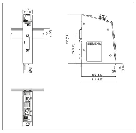
Figure 7-8 Dimension drawing of the Sensor Module Cabinet SMC20, all data in mm and (inches)
