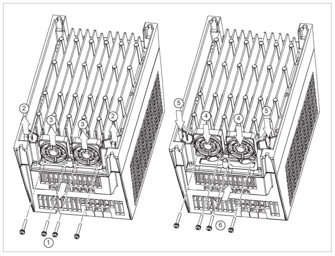
Figure 11-2 PM340 fan replacement, frame size FSB/FSC (0.4 Nm tightening torque)
