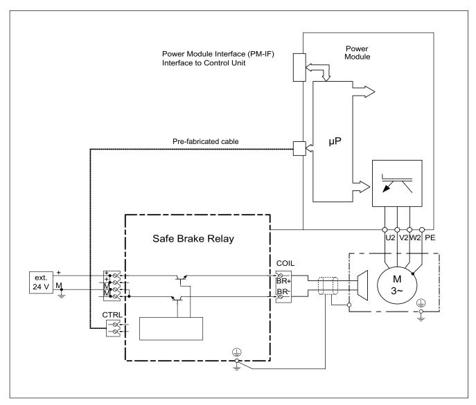
Figure 7-21 Safe Brake Relay connection example
