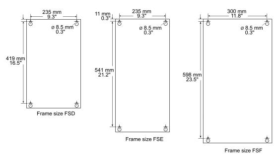
Figure 3-37 Hole drilling templates for frame sizes FSD to FSF
