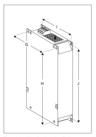
Figure 2-8 Mounting dimensions for line reactors with frame sizes FSB and FSC
