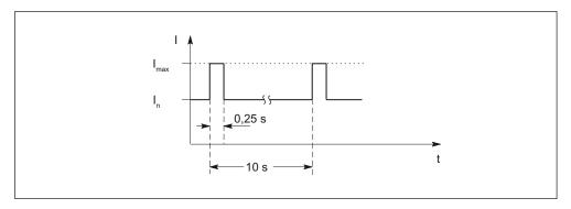
Figure 3-40 Duty cycle with initial load (for servo drives)
