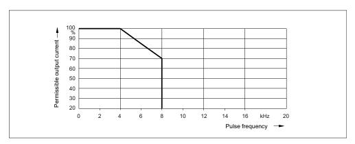
Figure 3-27 Frame size FSF: Output current as a function of the pulse frequency
