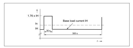
Figure 3-45 Duty cycle with 30 s overload with a duty cycle duration of 300 s
