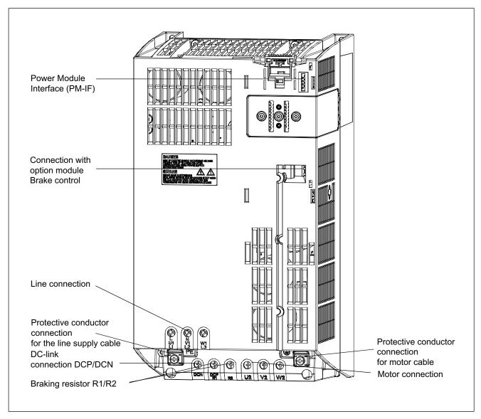
Figure 3-3 PM340, frame size FSC
