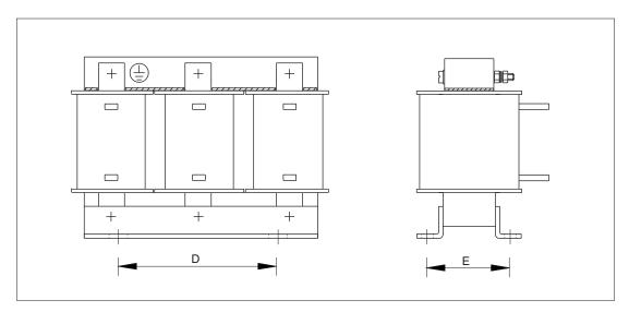
Figure 2-10 Mounting dimensions for line reactors with frame size FSF
