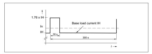
Figure 3-25 Duty cycle with 30 s overload with a duty cycle duration of 300 s
