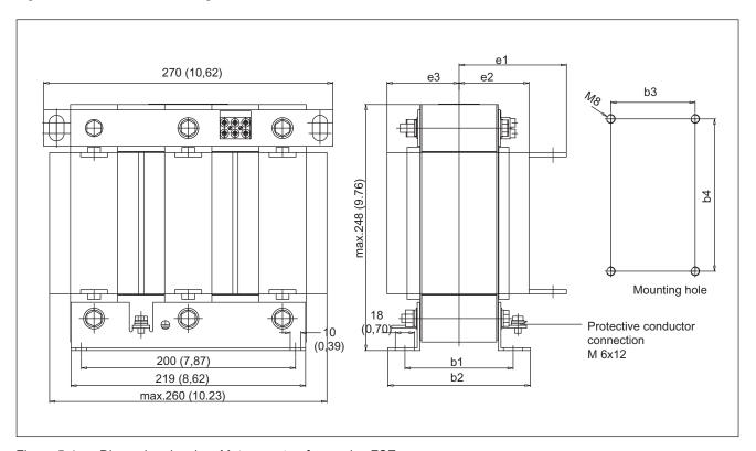
Figure 5-4 Dimension drawing: Motor reactor, frame size FSE
