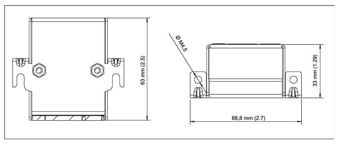
Figure 7-22 Dimension drawing of Safe Brake Relay, all data in mm and (inches)
