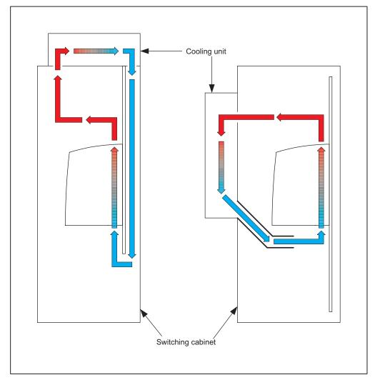
Figure 9-4 Examples of cabinet ventilation
