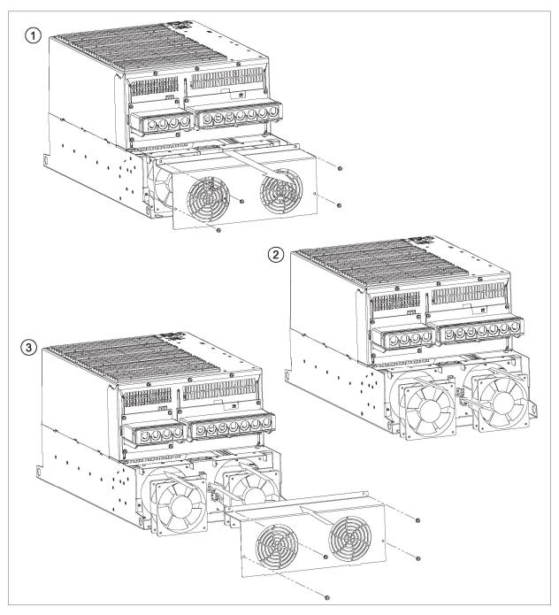
Figure 11-4 PM340 fan replacement, frame size FSF
