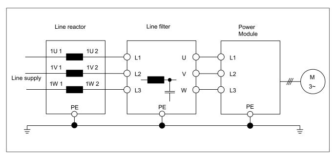
Figure 2-15 Power Module Blocksize with line reactor and line filter
