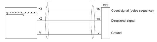
Figure 6-6 Connection of a pulse/direction interface with HTL level to interface X23
