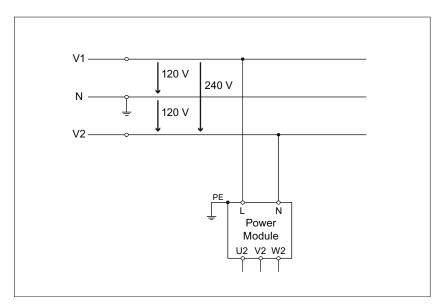
Figure 2-18 Direct operation on Single Phase Grounded Midpoint line system configuration
