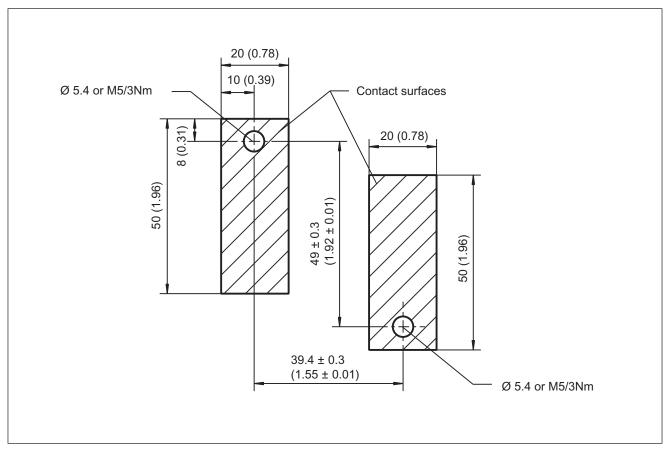
Figure 8-7 Hole drilling pattern for installation
