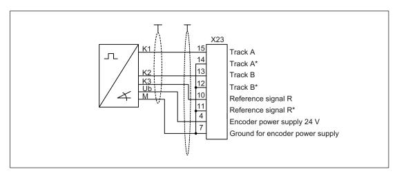
Figure 6-5 Connection example 2: HTL encoder, unipolar, with reference signal <sup>1)</sup>
