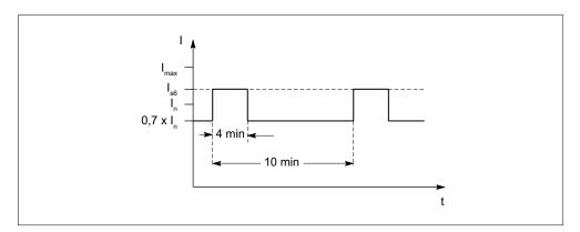
Figure 3-22 S6 duty cycle with initial load (for servo drives)
