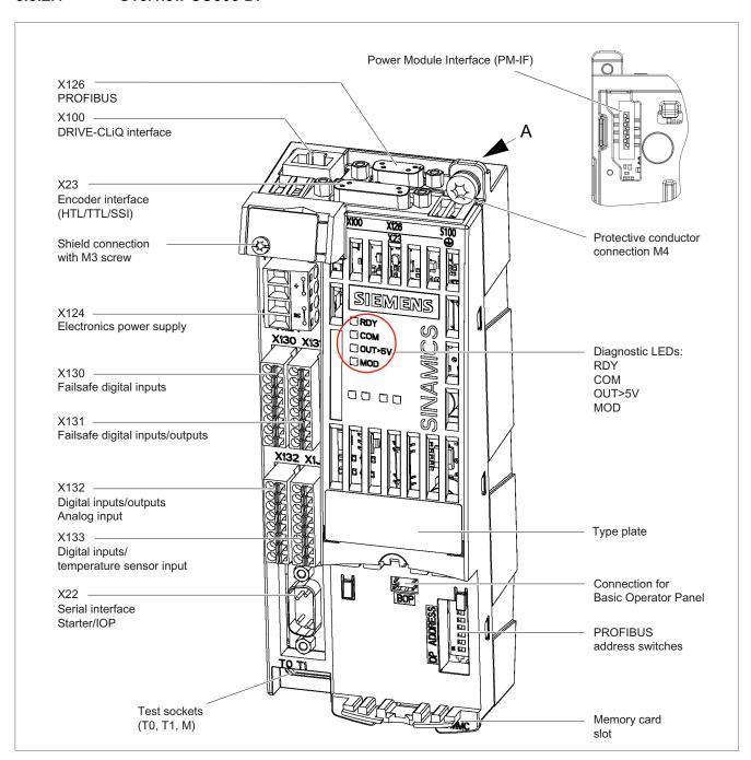
Figure 6-2 Description of the CU305 DP interfaces (ports)
