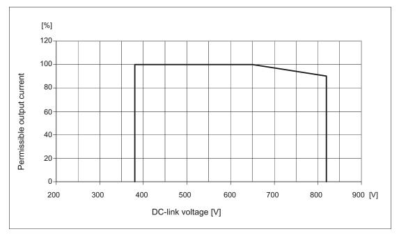
Figure 3-50 Current derating as a function of the DC-link voltage
