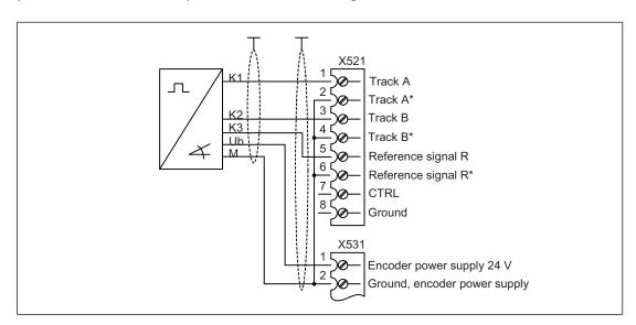
Figure 7-12 Connection example 2: HTL encoder, unipolar, with reference signal<sup>1)</sup>
