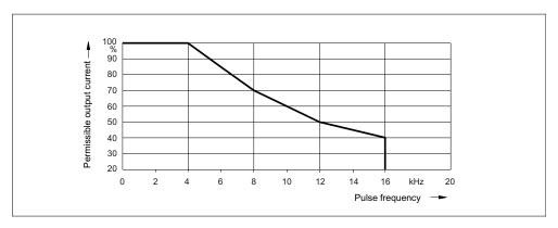
Figure 3-46 Frame sizes FSD and FSE: Output current as a function of the pulse frequency
