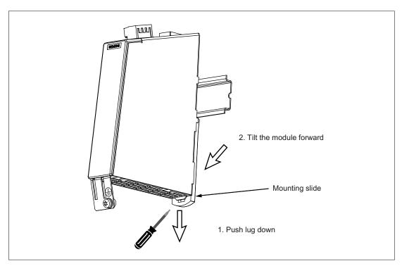
Figure 7-9 Removal of a component from a DIN rail
