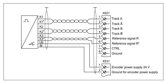
Figure 7-11 Connection example 1: HTL encoder, bipolar, with reference signal
