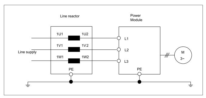
Figure 2-14 Power Module with line filter
