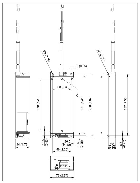
Figure 2-2 Dimension drawing of line filter, frame size FSA, all data in mm and (inches)
