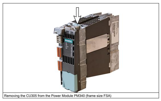
In order to remove the Control Unit from the Power Module, the blue release lever, as shown in the diagram, must be pressed downwards and the Control Unit swung out to the front.
