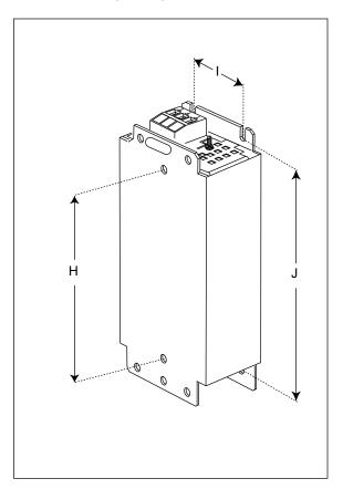
Figure 2-7 Mounting dimensions for line reactors with frame size FSA
