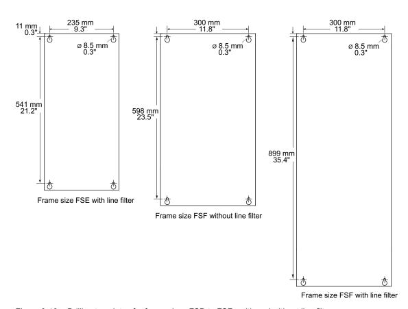
Figure 3-18 Drilling templates for frame sizes FSD to FSF - with and without line filter
