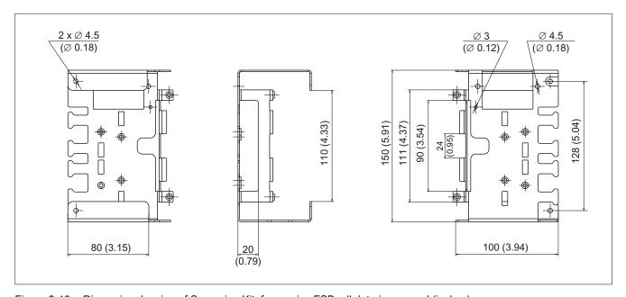
Figure 8-10 Dimension drawing of Screening Kit, frame size FSB, all data in mm and (inches)
