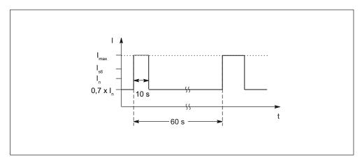
Figure 3-43 Duty cycle with initial load (for servo drives)
