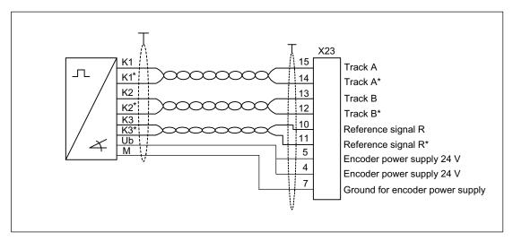
Figure 6-4 Connection example 1: HTL encoder, bipolar, with reference signal
