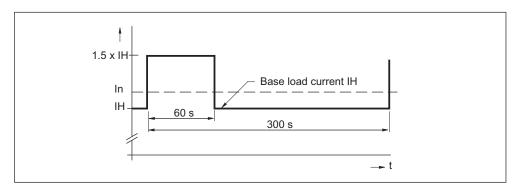
Figure 3-44 Duty cycle with 60 s overload with a duty cycle duration of 300 s
