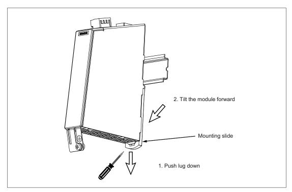
Figure 7-15 Removal of a component from a DIN rail
