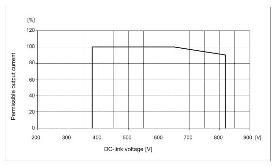
Figure 3-30 Current derating as a function of the DC-link voltage
