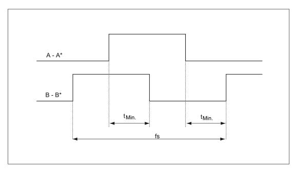
Figure 7-18 Signal characteristic of track A and track B between two edges: Time between two edges with pulse encoders
