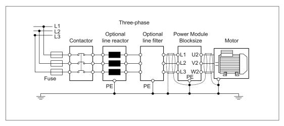
Figure 2-1 Example of a line connection for Power Modules blocksize with no integrated line filter
