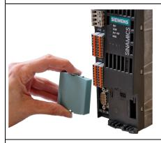
3. To remove the blanking cover, press the latching cams of the cover together simultaneously and pull the cover straight out.
