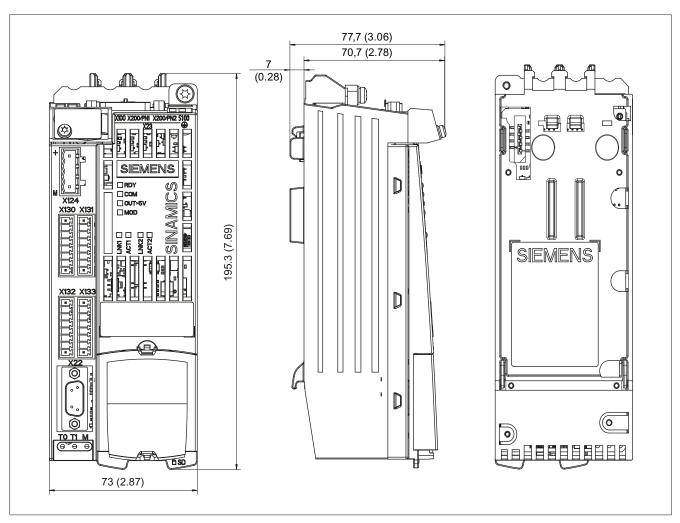
Figure 6-13 Dimension drawing of Control UnitCU305 PN, all data in mm and (inches)
