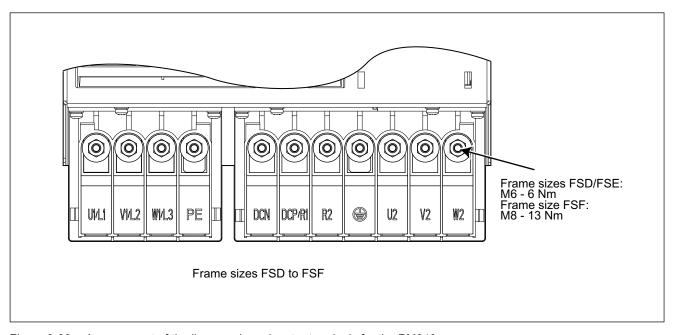
Figure 3-33 Arrangement of the line supply and motor terminals for the PM340
