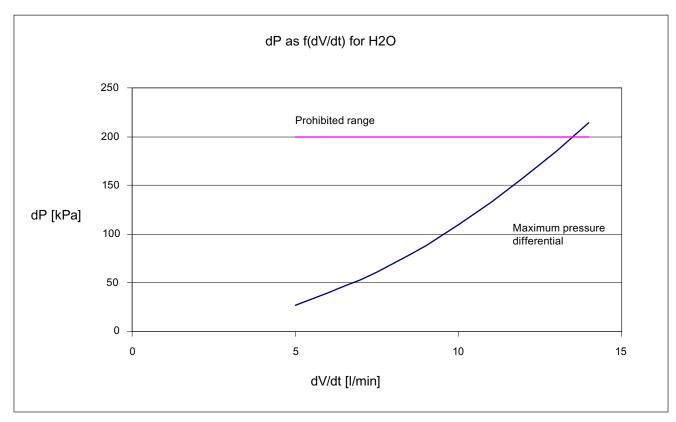
Figure 10-3 Pressure difference as a function of volumetric flow
