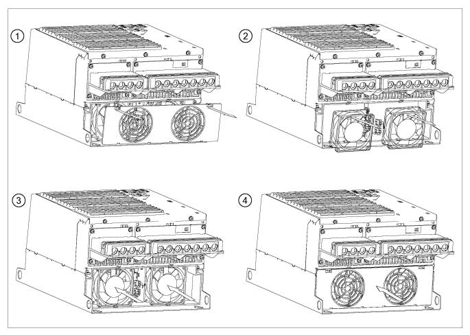
Figure 11-3 PM340 fan replacement, frame sizes FSD/FSE
