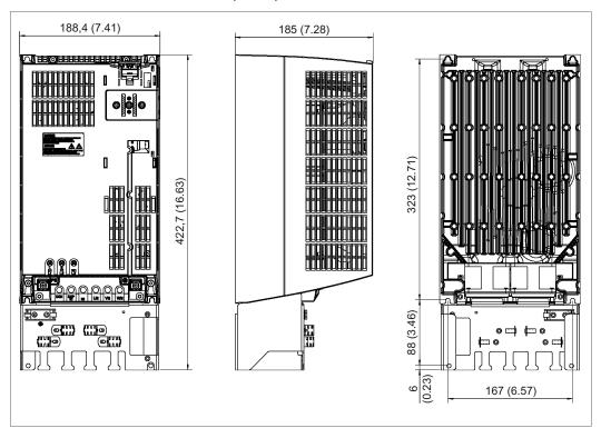
Figure 8-14 Dimension drawing of PM340 Power Module with Screening Kit, frame size FSC, all dimensions in mm and (inches)
