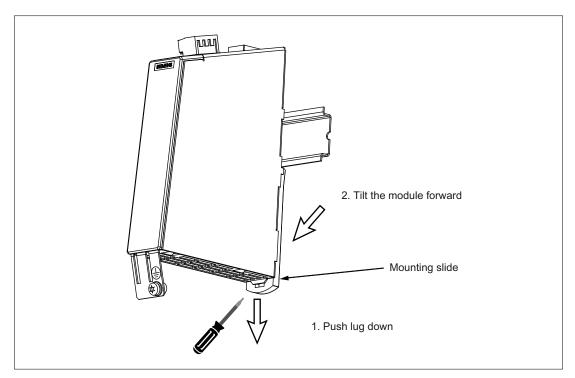
Figure 7-5 Removal of a component from a DIN rail
