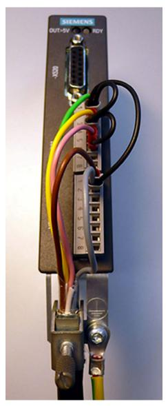
Figure 7-13 Photo of connection example 2: SMC30, 30 mm wide
