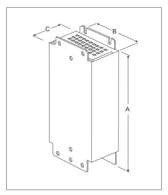
Figure 5-1 Dimension drawing: Motor reactor, frame size FSA
