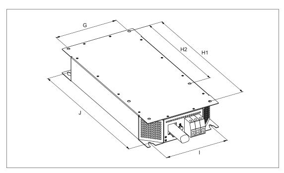
Figure 2-9 Mounting dimensions for line reactors with frame sizes FSD and FSE
