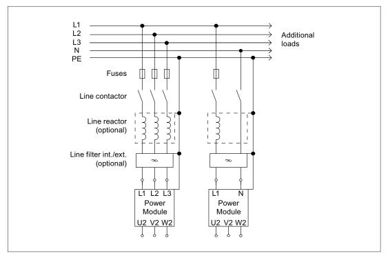
Figure 2-17 Direct operation on the line supply
