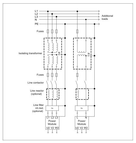
Figure 2-20 Isolating transformer
