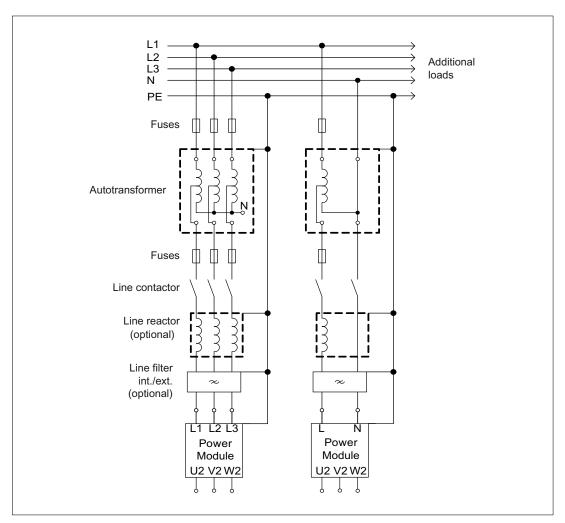
Figure 2-19 Autotransformer
