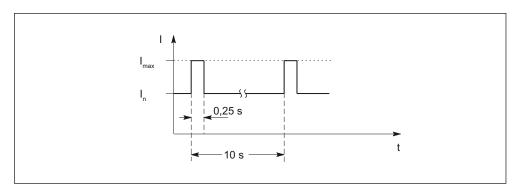
Figure 3-20 Duty cycle with initial load (for servo drives)
