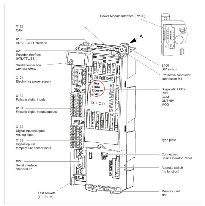
Figure 6-3 Interface description CU305 CAN
