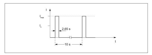
Figure 3-41 Duty cycle without initial load (for servo drives)
