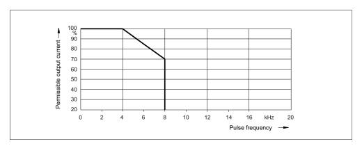
Figure 3-47 Frame size FSF: Output current as a function of the pulse frequency
