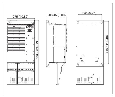
Figure 8-15 Dimension drawing of PM340 Power Module with Screening Kit, frame size FSD, all dimensions in mm and (inches)
