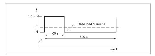
Figure 3-24 Duty cycle with 60 s overload with a duty cycle duration of 300 s
