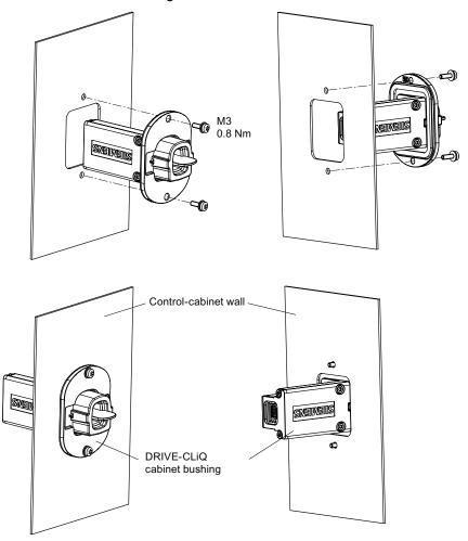
Figure 8-4 Installing the DRIVE-CLiQ cabinet bushing
