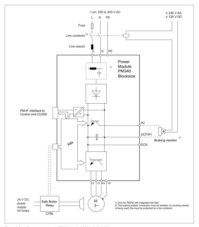
Figure 3-8 Connection example PM340, 1-ph. 200 V - 240 V AC
