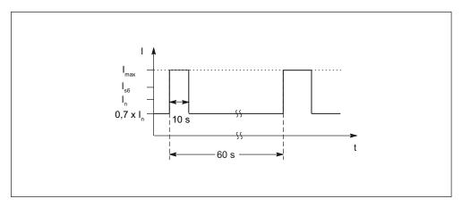
Figure 3-23 Duty cycle with initial load (for servo drives)
