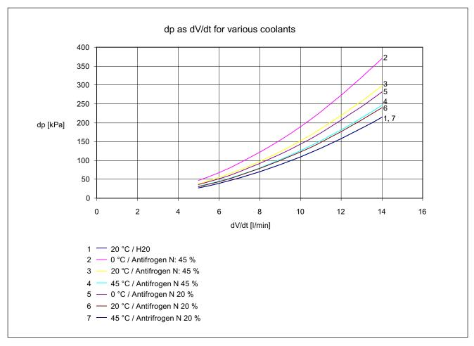
Figure 10-4 Pressure difference as a function of volumetric flow for various coolants and temperatures
