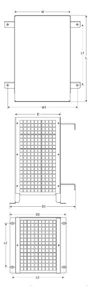
Figure 4-4 Dimension drawing of braking resistor, frame sizes FSC, FSD, FSE, FSF
