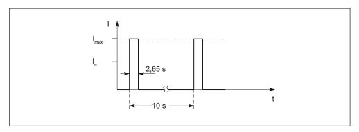
Figure 3-21 Duty cycle without initial load (for servo drives)
