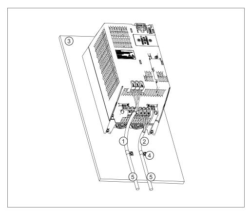
Figure 9-1 Shielding of a Power Module PM340
