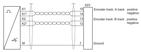
Figure 6-7 Connection of TTL encoders to interface X23 for setpoint value specification via A track and B track
