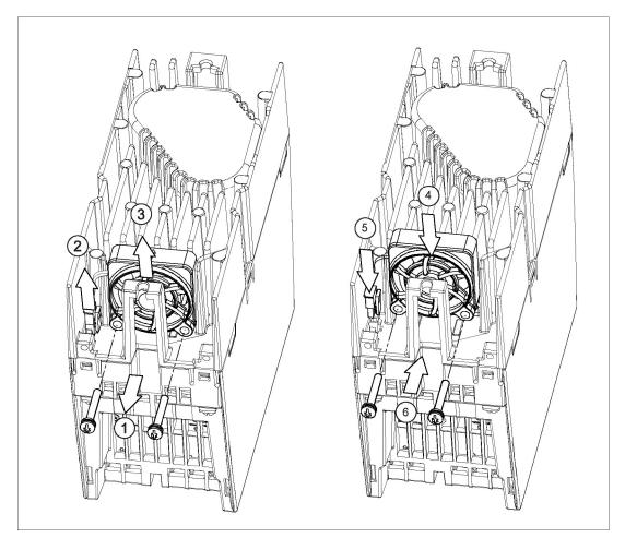
Figure 11-1 PM340 fan replacement, frame size FSA
