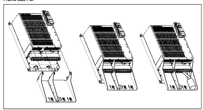
Figure 8-24 Mounting a Screening Kit on a Liquid Cooled Power Module PM340, frame size FSF
