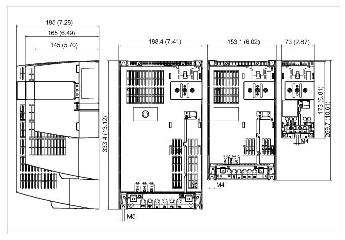
Figure 3-10 Dimension drawings, Power Module PM340
