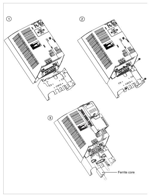
Figure 8-19 Mounting a Screening Kit and ferrite core on a Power Module of frame sizes FSB and FSC
