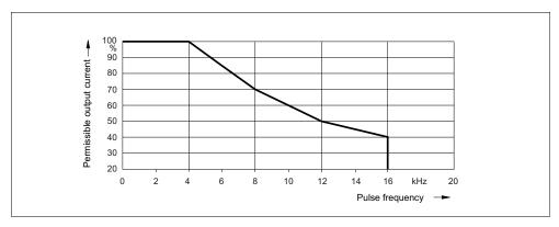
Figure 3-26 Frame sizes FSA to FSE: Output current as a function of the pulse frequency
