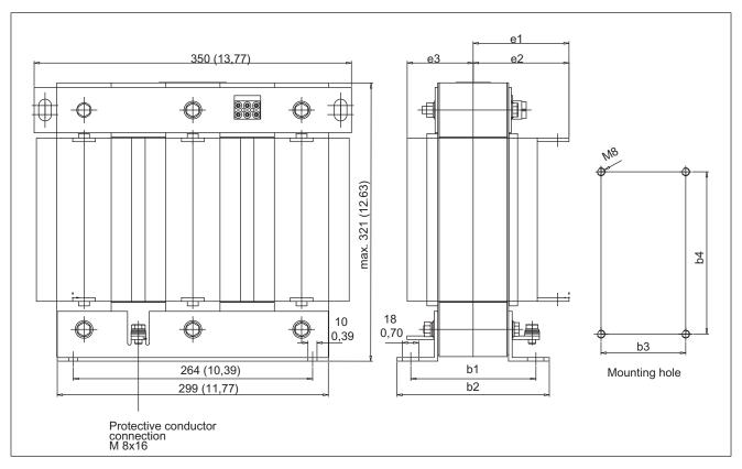
Figure 5-5 Dimension drawing: Motor reactor, frame size FSF
