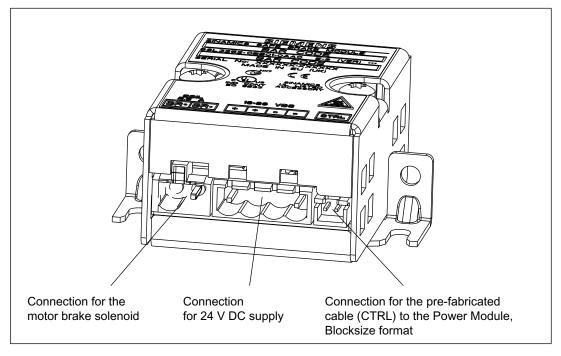
Figure 7-20 Interface description: Safe Brake Relay
