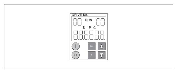
Figure 7-2 Overview of displays and keys
