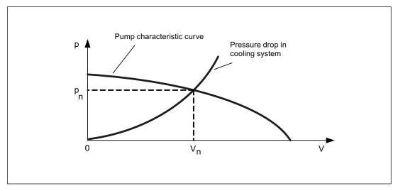
Figure 10-2 Pump characteristic curve
