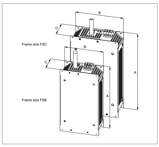
Figure 5-2 Dimension drawing: Motor reactor, frame sizes FSB and FSC
