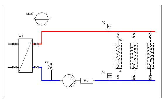
Figure 10-1 Example of a closed cooling circuit
