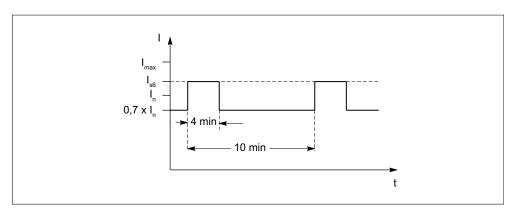
Figure 3-42 S6 duty cycle with initial load (for servo drives)
